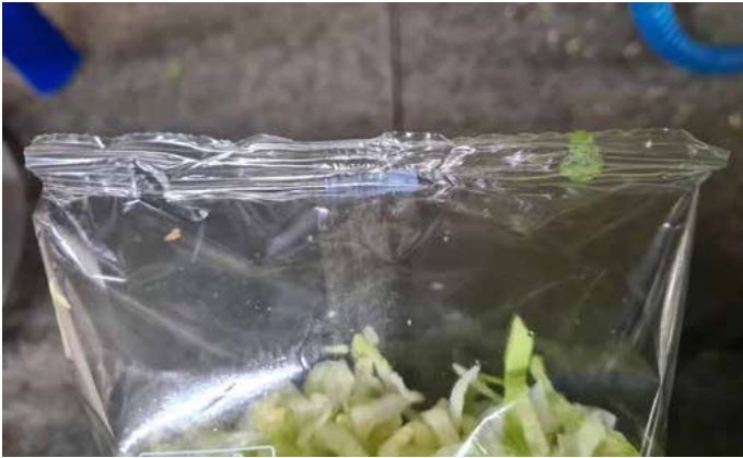
The QipScan measures each deviation in the seal, such as product that is trapped or heat transmission failures during welding of a seal.
